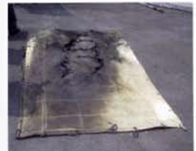
No piercing of BlastMat.
