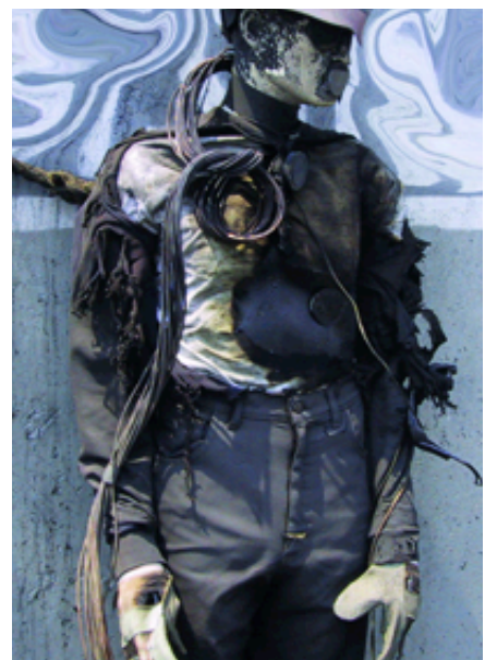
Unprotected mannequin after a chest level arc blast.
